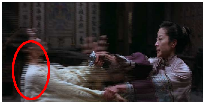
Fig. 2. Line-crawling effect occurs when merged directly.
