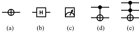
Fig. 2. Symbols for (a) N, (b) H, (c) measurement, (d) CN, and (e) CCN gates.
