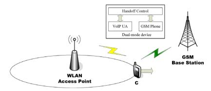
Fig. 7. Dual-mode communication.
