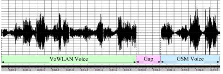
Fig. 10. Audio gap during VoWLAN-to-GSM handoff.
