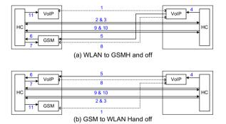
Fig. 8. Vertical handoff procedure on the dual-mode handset.
