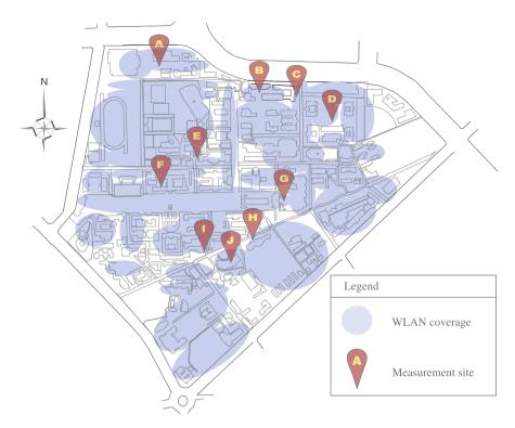
Fig. 2. NTU campus WLAN coverage.
