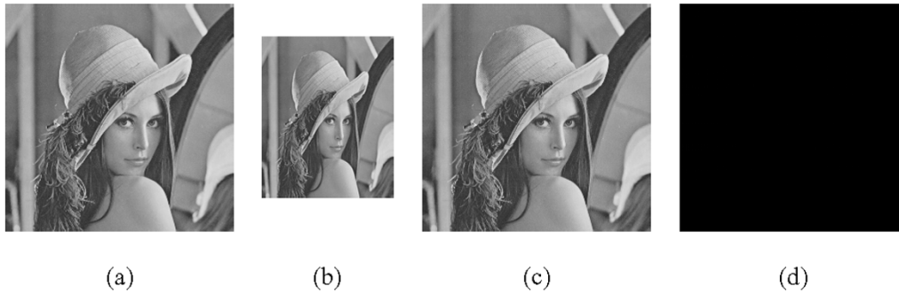
Fig. 4. (a) Original input image. (b) Down sampled image in the upper channel. (c) Perfectly reconstructed output image. (d) Reconstruction error.
