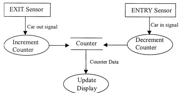
Fig. 10 Functional model of a DISPLAY subsystem.
