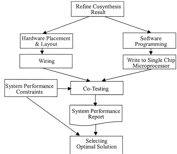
Fig. 7 Emulation flow diagram.
