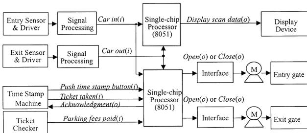
**Fig. 13** Block diagram for prototype  $\mathbf{D}(S_C, H_S, S_M)$ .
