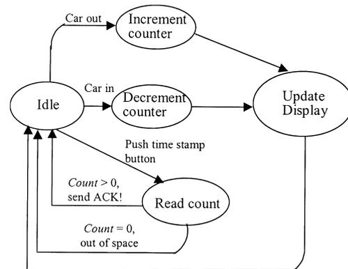
Fig. 9 Dynamic model of a DISPLAY subsystem.
