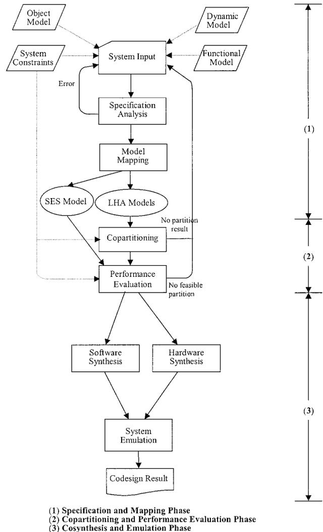
Fig. 1 Distributed embedded system codesign methodology.
