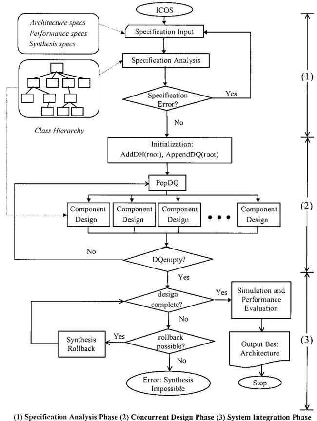
Fig. 6 Hardware synthesis flow (ICOS [2]).
