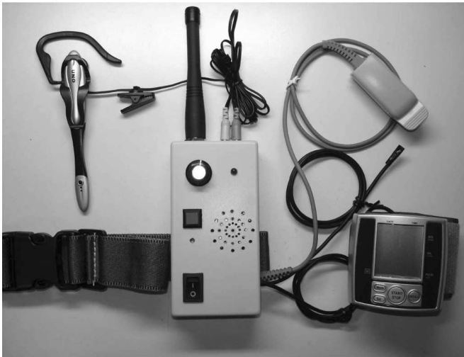
Fig. 3. Photograph of the mobile physiological examination device.
