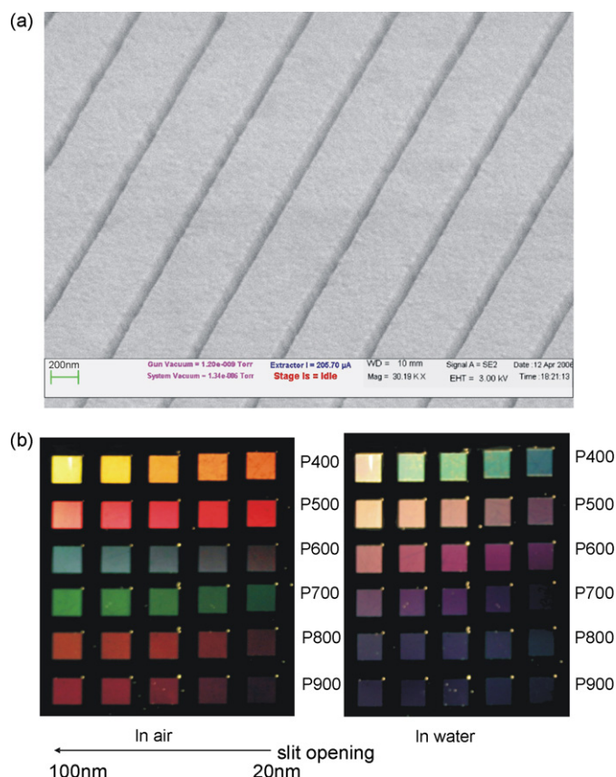
Fig. 1. (a) The SEM image of a gold nanoslit array. The array had a period of 600 nm and the slit width was about 80 nm. (b) The transmission optical images of various nanoslit arrays in air and in water environment. The array period changed from 400 nm to 900 nm and slit width, from 20 nm to 100 nm. The area of each nanoslit array was 150\mu\text{m} \times 150\mu\text{m} . The colors of the nanoslit arrays are due to extraordinary transmissions of surface plasmon resonances.
