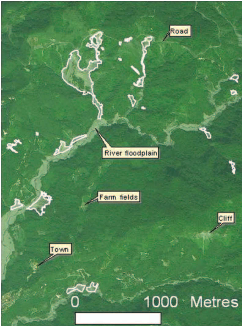
Figure 3. Delineated landslides (white outline) in 2.5 m SPOT-5 imagery.
