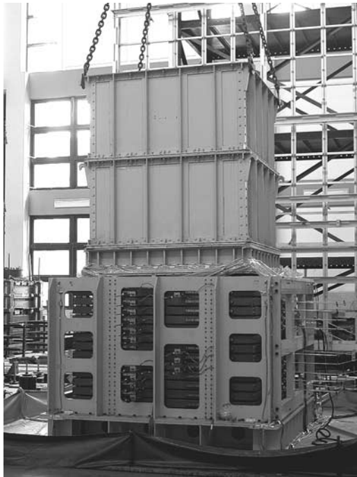
FIG. 4—Specimen preparation with the pluviator.
