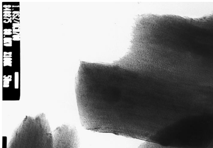
Fig. 5. Transmission electron micrograph of SZA/MCM-41 calcined at 700°C for 3 h. Zr(SO_4)_2/MCM-41 ratio = 1.0 (g/g); Al content = 0.3 wt.%.
