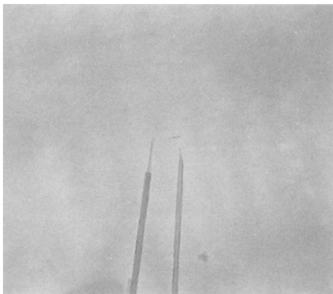
FIG 4 Transmission electron micrograph of a carbon nanotube after reaction with O_3 for 12 h.
