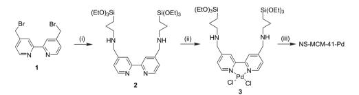
Scheme 2. Preparation of NS-MCM-41-Pd: (i)  $H_2N(CH_2)_3Si(OEt)_3$ ,  $Et_3N$ , THF, 50 °C, 6 h; (ii)  $PdCl_2(PhCN)_2$ , toluene, rt and (iii) NS-MCM-41, toluene, reflux, 48 h, then  $Me_3SiCl$ , 70 °C.
