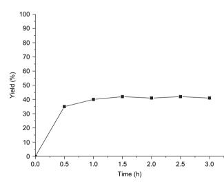
Figure 2. Plot of yields versus time for the hot-filtration experiment. The NS-MCM-41-Pd was filtered off after 0.5 h reaction at 50 °C.  $[C_6H_5I]/[4-CH_3OC_6H_4MgBr]/[Pd]=500/625/1$ .
