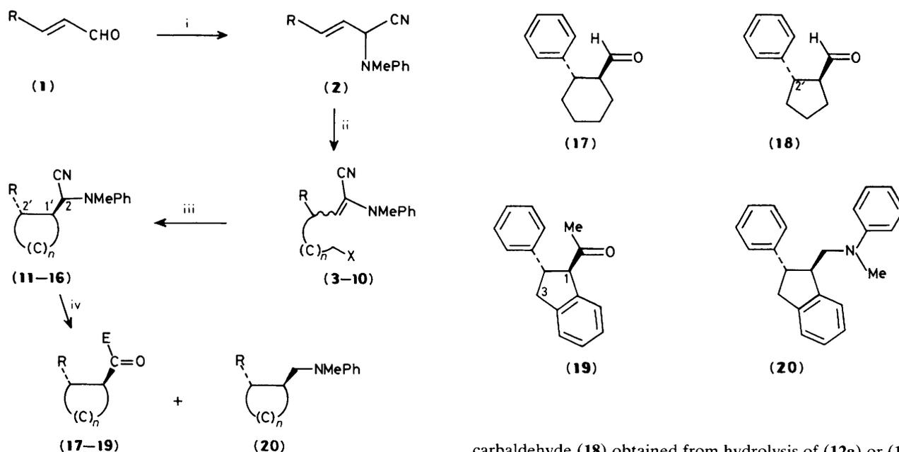
**Scheme 1.** Reagents and conditions: i, PhMeNH<sub>2</sub><sup>+</sup>Cl<sup>-</sup>, Et<sub>2</sub>O, KCN, H<sub>2</sub>O, 0 °C, 2 h; ii, LDA (Bu<sup>t</sup>OK), dihalide, -78 °C (0 °C), 1–2 h; iii, Bu<sup>n</sup><sub>3</sub>SnH, AIBN cat., PhH, 80 °C; iv, for alkylation: LDA, THF, halide (excess), -78 °C to room temperature; for hydrolysis: CuSO<sub>4</sub>, H<sub>2</sub>O, MeOH, 0 °C, 3 h; for reductive decyanation: NaBH<sub>4</sub>, EtOH, 30 °C, 20 h.
