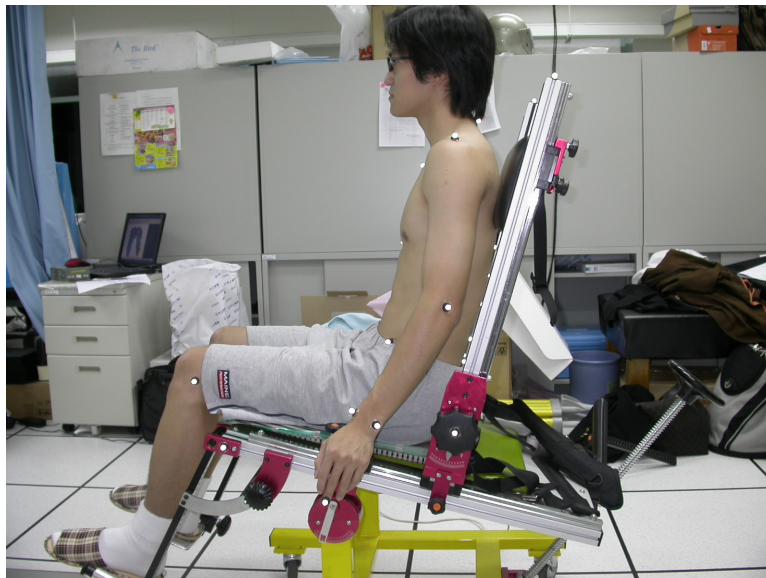
Figure 1. The subject sit on an adjustable chair which may change the seat depth, the height of foot pad, and seat tilt-angle. The markers were placed on the subject, pressure plate, and chair.
