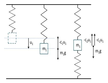
Figure 4.1: The left one is a spring without any mass. The middle one is a spring hanging a mass  $m_1$  freely. The right one is a mass  $m_1$  with two springs fixed on the ceiling and floor.
