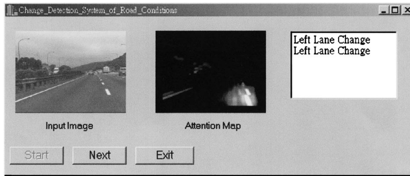
Fig. 11. Visual interface for reporting the results of change detection in driving environment.
