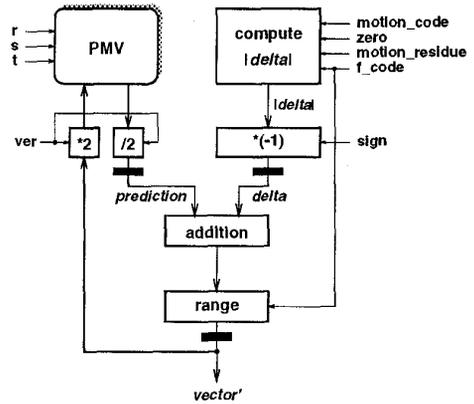
Figure 3: Architecture of motion vector decoder.
