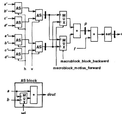
Figure 4: Architecture of Predicted picture reconstructor.
