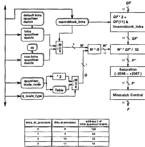
Figure 2: Architecture of inverse quantization.
