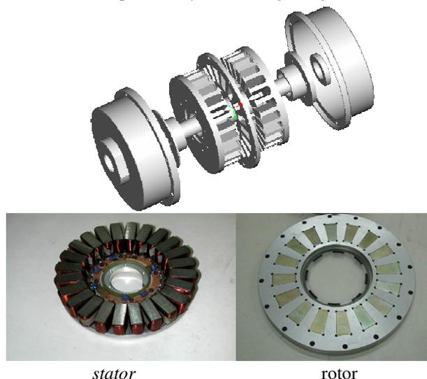
Fig. 1. Wheel motor assembly, stator and rotor.
