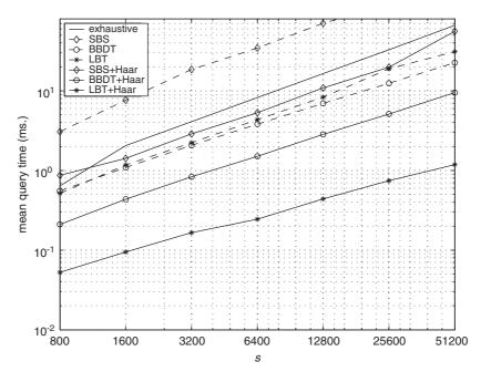
Fig. 6. Mean query time versus size, s, of the sample point set (d = 32).
