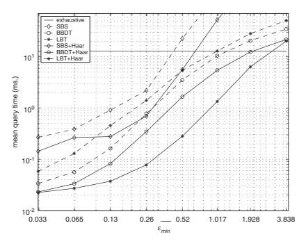
Fig. 8. Mean query time versus mean of the minimum distances,  $\overline{\varepsilon_{min}}$  (s = 10,000, d = 32).
