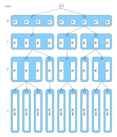
Fig. 2. An example of hierarchical construction of the LB-tree. All the points in the same dark region are determined agglomeratively and are grouped into a cluster. Notice that each point is transposed in order to fit into the limited space.
