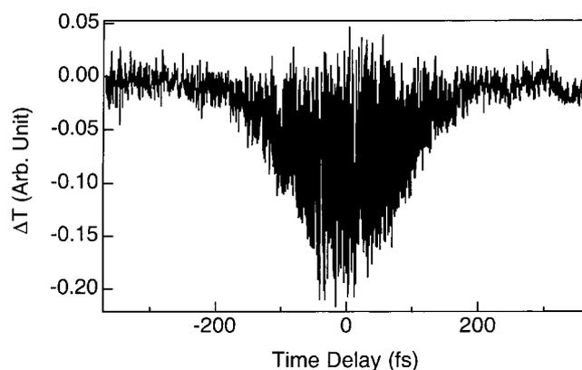
Fig. 1. Single-scan autocorrelation trace for 720 nm IR pulses measured in a GaN thin film with a sapphire substrate.
