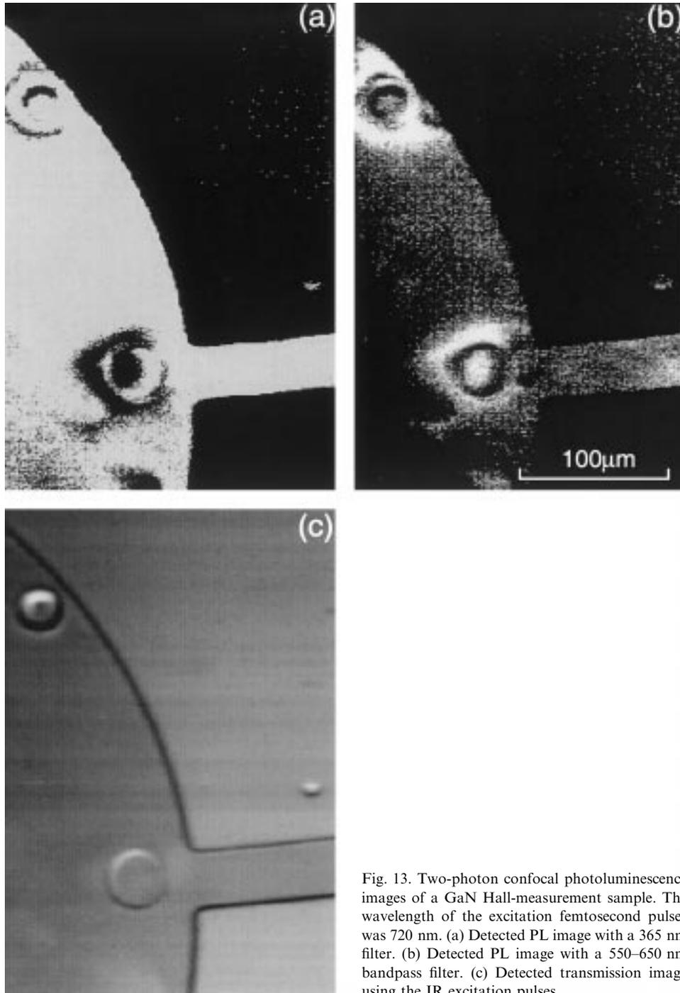
Fig. 13. Two-photon confocal photoluminescence images of a GaN Hall-measurement sample. The wavelength of the excitation femtosecond pulses was 720 nm. (a) Detected PL image with a 365 nm filter. (b) Detected PL image with a 550–650 nm bandpass filter. (c) Detected transmission image using the IR excitation pulses.
