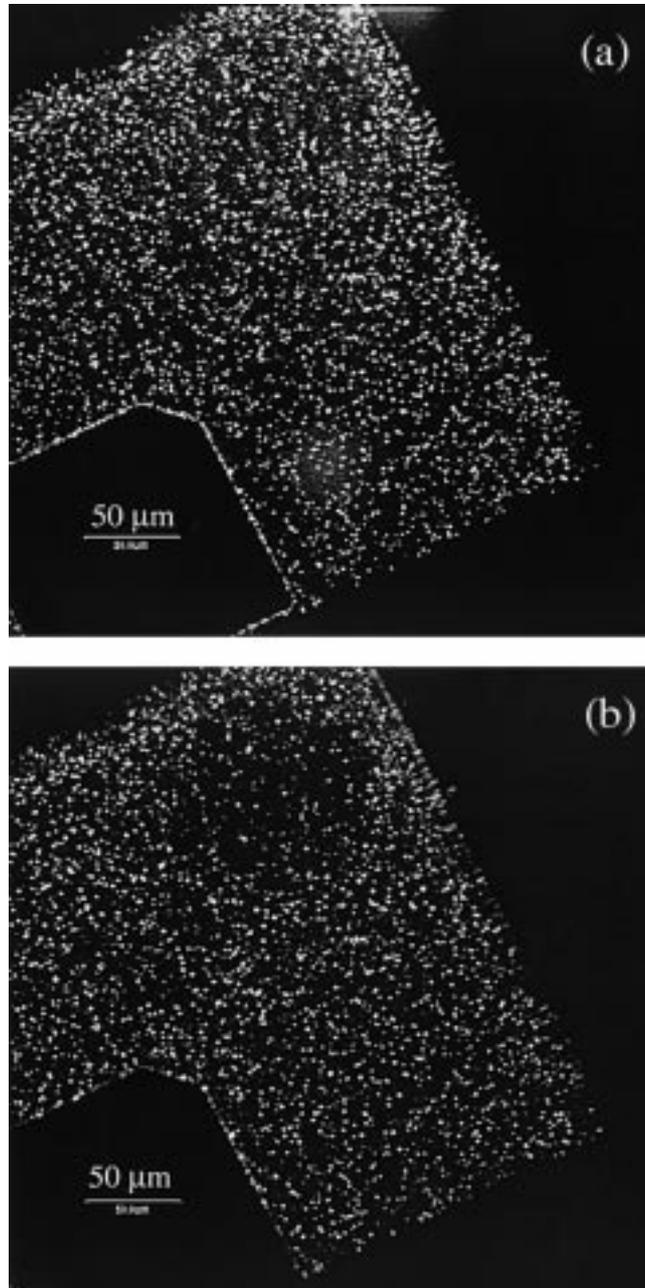
Fig. 14. (a) Two-photon PL image and (b) two-photon OBIC image of a green InGaN/GaN LED. The excitation wavelength was 760 nm. A green filter was used in the PL image.
