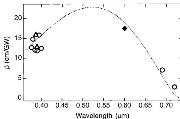
Fig. 6. Measured TPA coefficient versus wavelength. Open circles represent the values obtained from TPA autocorrelation measurements. Open triangles represent the values obtained from Z-scan measurements. Previously reported value from Petit *et al.* (1997) is also displayed as a solid diamond for comparison. Dotted line is 12 times of Equation (2).
