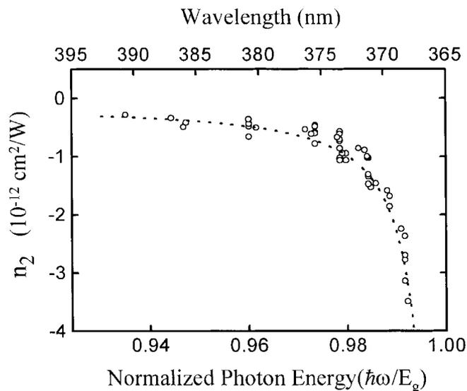
Fig. 12. Measured nonlinear refractive index (open circles) versus wavelength. The dotted line is a reference curve governed by quadratic Stark and two-photon absorption effects.
