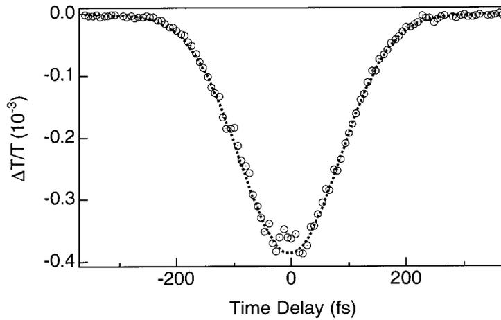
Fig. 3. Multiple-scan autocorrelation trace for 720 nm IR pulses measured by TPA-induced transmission changes in a GaN thin film.
