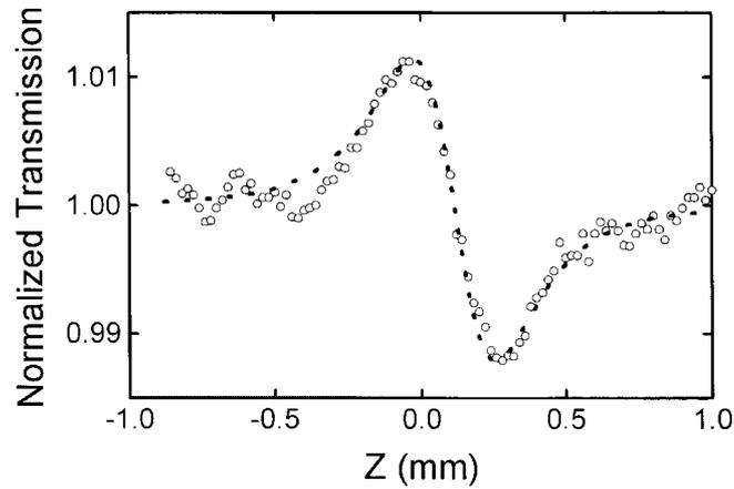
Fig. 10. Small aperture Z-scan trace of GaN measured at 375 nm. The dotted line is a fitting curve.
