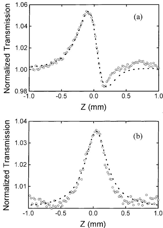
Fig. 8. (a) Small aperture Z-scan trace of GaN measured at 369 nm. The dotted line is a fitting curve with a beam diameter of 10  $\mu\text{m}$ . (b) Open aperture background signal at 369 nm and its fitting curve.
