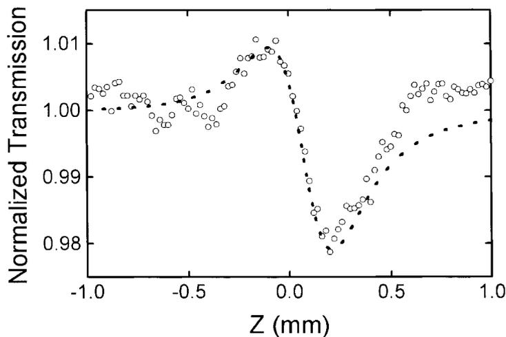
Fig. 11. Small aperture Z-scan trace of GaN measured at 387 nm. The dotted line is a fitting curve.
