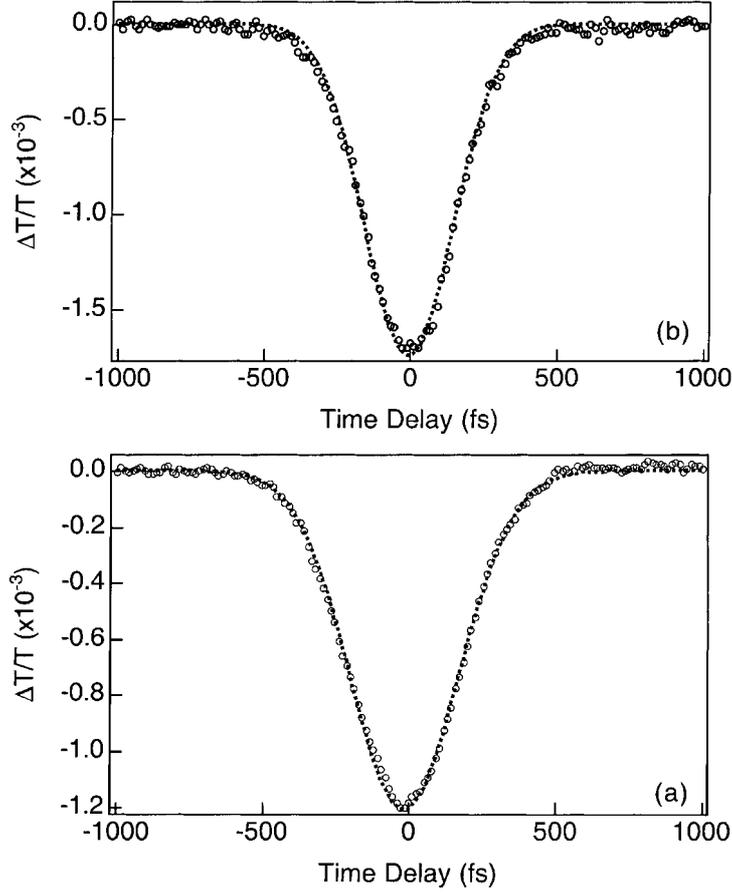
Fig. 5. (a) Measured TPA autocorrelation trace after modification at 390 nm wavelength. (b) Measured TPA autocorrelation trace after modification at 380 nm wavelength.
