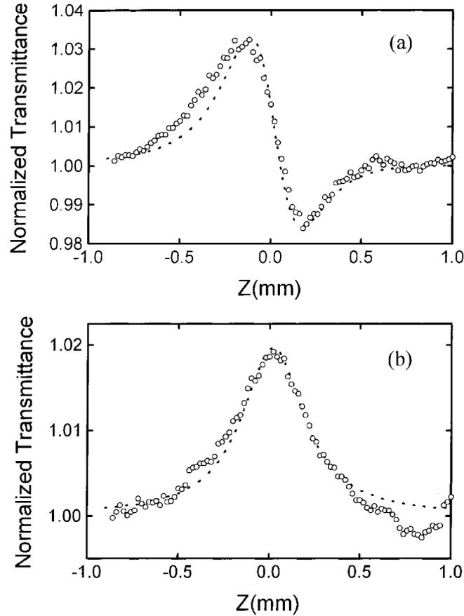
Fig. 7. (a) Small aperture Z-scan trace of GaN measured at 371 nm. The dotted line is a fitting curve with a beam diameter of 10  $\mu\text{m}$ . (b) Open aperture background signal at 371 nm and its fitting curve.
