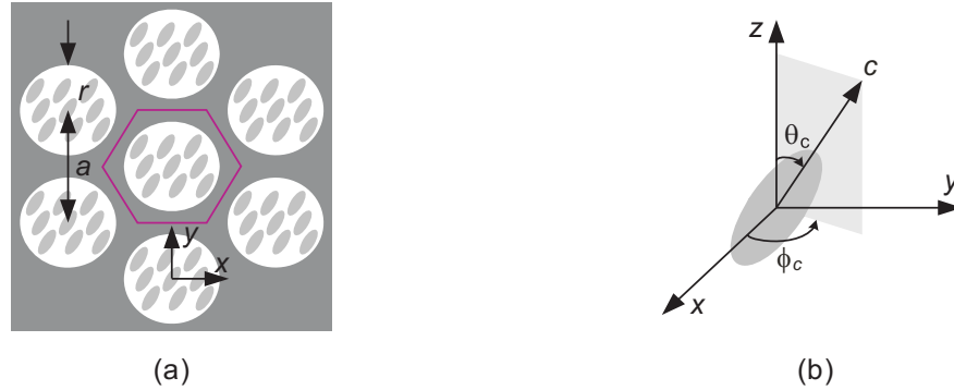
Fig. 7. (a) Cross-section of the 2D anisotropic PC with triangular lattice. (b) Schematic definition of rotation angles for the LC molecule.
