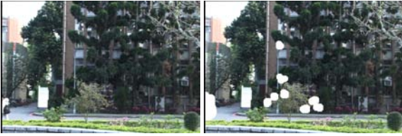
Figure 6: Left: The frame after aligning to the stabilized camcorder motion path. Right: The mask of detected moving objects (white regions).
