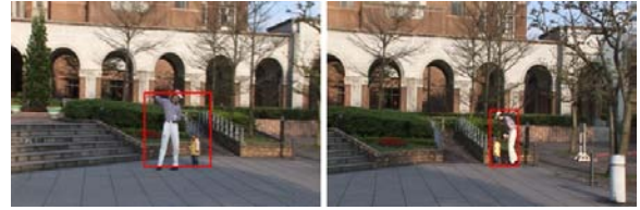
Figure 3: The detected moving objects.
