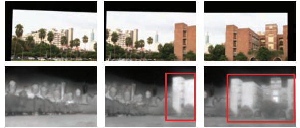
Figure 5: Top row: Aligned frames of the top row of Figure 2 without considering video ROI. The black regions show the missing areas and the building is cut out. Bottom row: The saliency maps of the top row of Figure 2.
