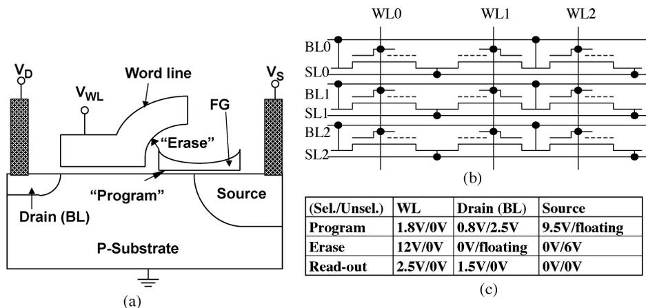
Fig. 1. (a) Cross section of the split-gate cell under study. (b) Memory array schematic diagram. (c) Typical cell operation conditions.
