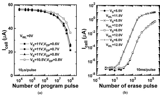
Fig. 2. (a) Program disturb:  $I_{cell}$  versus programming times under different programmed drain ( $V_{DP}$ ) and source ( $V_S$ ) voltage. The WL voltage ( $V_{WL}$ ) is 0 V and the pulsewidth is 10  $\mu s$  for all conditions. (b) Erase disturb: under different WL and inhibited source voltages. The pulsewidth is 10 ms.
