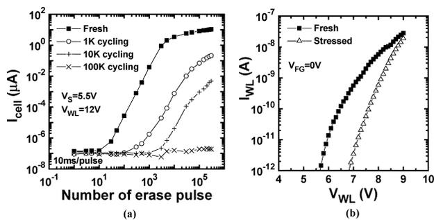
Fig. 3. (a) Erase disturb performance for the cell under different P/E cycles. The disturb testing condition is 12-V WL voltage and 5.5-V inhibited source voltage. (b) The voltage of the stressed tunnel oxide at 1-pA tunneling current shows 1.1-V less than that of fresh tunnel oxide. The  $I$ - $V$  current is taken from the FG-connected cell mini-array.
