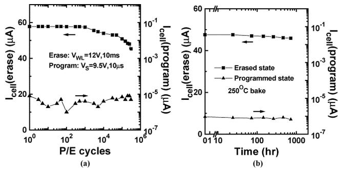
Fig. 4. (a) P/E cycling endurance test can pass 300 k times. (b) The data retention result for the cells after 300-k P/E cycling stress. The baking temperature is 250 °C.
