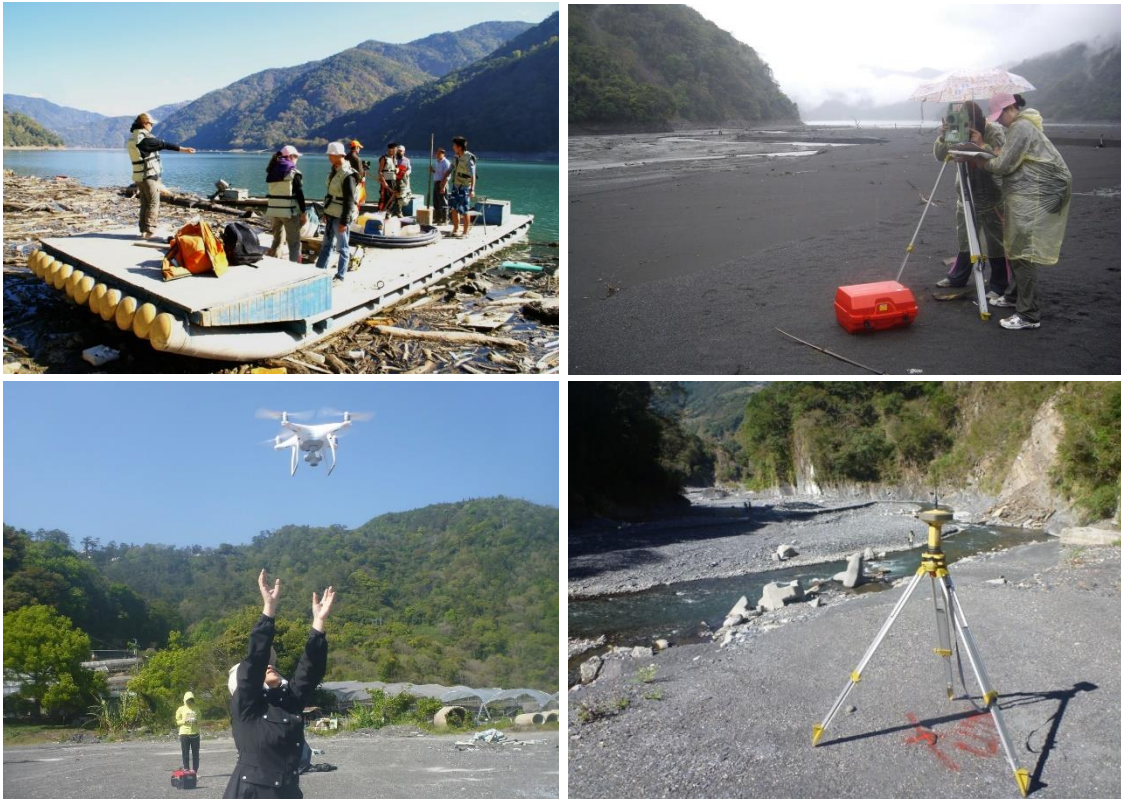
Fig. 3: Tools used for the repeat survey campaigns. Top left, boat used to survey the reservoir bathymetry. Top right, total station used to acquire topography transects. Bottom left, UAV used to acquire high resolution orthophotos and DTMs of the delta surface. Bottom right, GPS station used to position ground controls.
