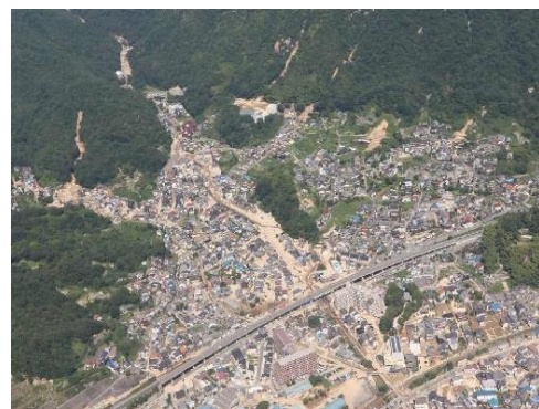
Photo 1.3 Sediment runoff and flooding due to torrential rain in July 2018 (Kure, Hiroshima Prefecture) 1)
