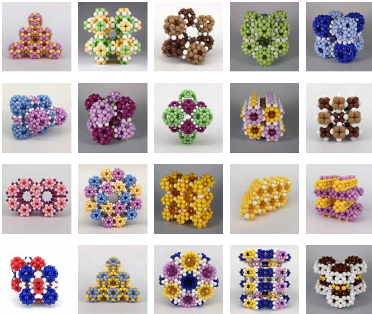
Figure 4: Zeolites specified by 3-letter Framework Type Codes. First row: SOD (Sodalite), LTA, FAU, EMT, RHO; Second row: KFI, AST, TSC, ATN, BCT; Third row: LTL, MOZ, SAS, ABW, BEC; Fourth row: MEP, MTN, DOH, MWW (MCM-22), SSF.
