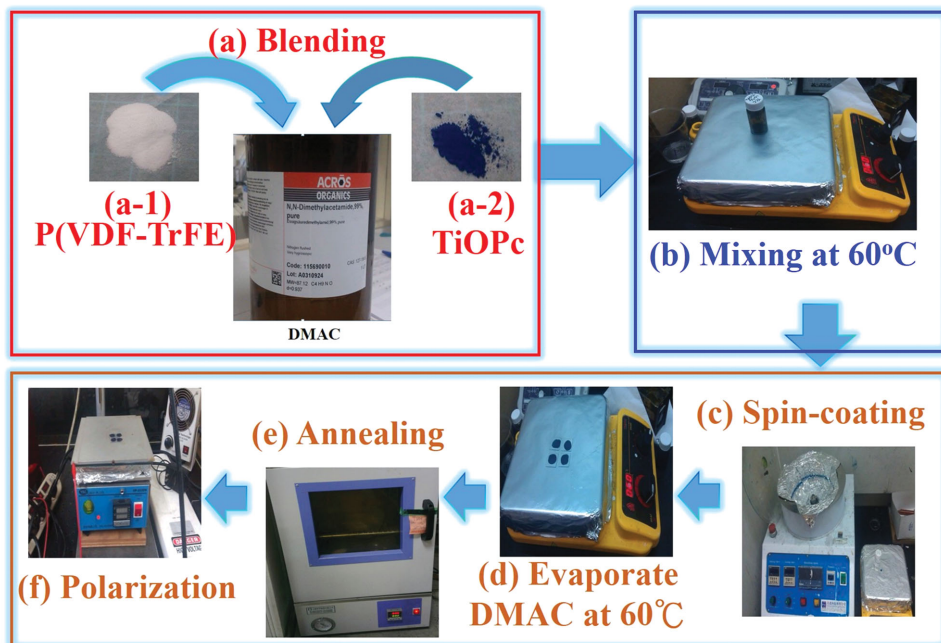
Figure 2. Sample-preparation procedures: a) Blending (a-1) poly(vinylidene fluoride-co-trifluoroethylene) (P(VDF-TrFE)) with (a-2) titanium oxide phthalocyanine (TiOPc) powders. b) Mixing the composite at 60 °C. c) Spin-coating the composed film on a PET plate with an ITO electrode. d) Heating the sample to evaporate dimethylacetamide (DMAC) solvent. e) Annealing the sample in a 100 °C vacuum oven for six hours. f) Polarizing the samples.
