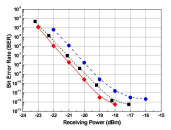
Fig. 10. BER performance of the back-to-back NRZ (blue circle) and the TWSOA converted RZ under DFBLD (black square) and FPLD (red diamond) based inverse-optical-comb injection.
