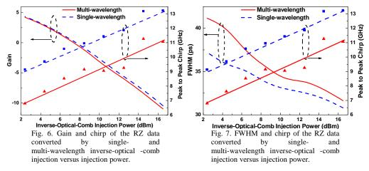
To provide a fast conversion speed and shortened response, the increase in both the biased current of the TWSOA and the injection power of inverse-optical-comb are mandatory. Nonetheless, the shortening of converted RZ pulsewidth inevitably results in a large dynamic frequency chirp under a same gain depletion depth of TWSOA. The increasing trend of the peak-to-peak dynamic frequency chirp with increasing gain of TWSOA (see Fig. 8) is plot
