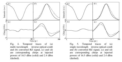
Theoretically, the gain coefficient of TWSOA exhibits a Lorentzian lineshape described determined by both the pumped carrier concentration and the spectral distribution [12], as described in Eq. (2). The RZ data-format conversion occurred in TWSOA under the intense cross-gain depletion process not only results in patterning effect in time domain, but also induces a large chirp with its level proportional to the depth of gain depletion. Nonetheless,
