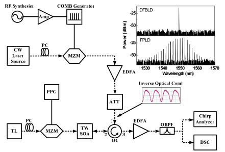
Fig. 1. Experimental setup. Amp.: amplifier.; ATT.: optical attenuator; DSO: digital sampling oscilloscope; EDFA: erbium doped fibre amplifier; OBPF: optical band-pass filter; OC: optical circulator; PC: polarization controller; PPG: PRBS pattern generator; TL: tunable laser. Electrical path: solid line. Optical path: dash line.
