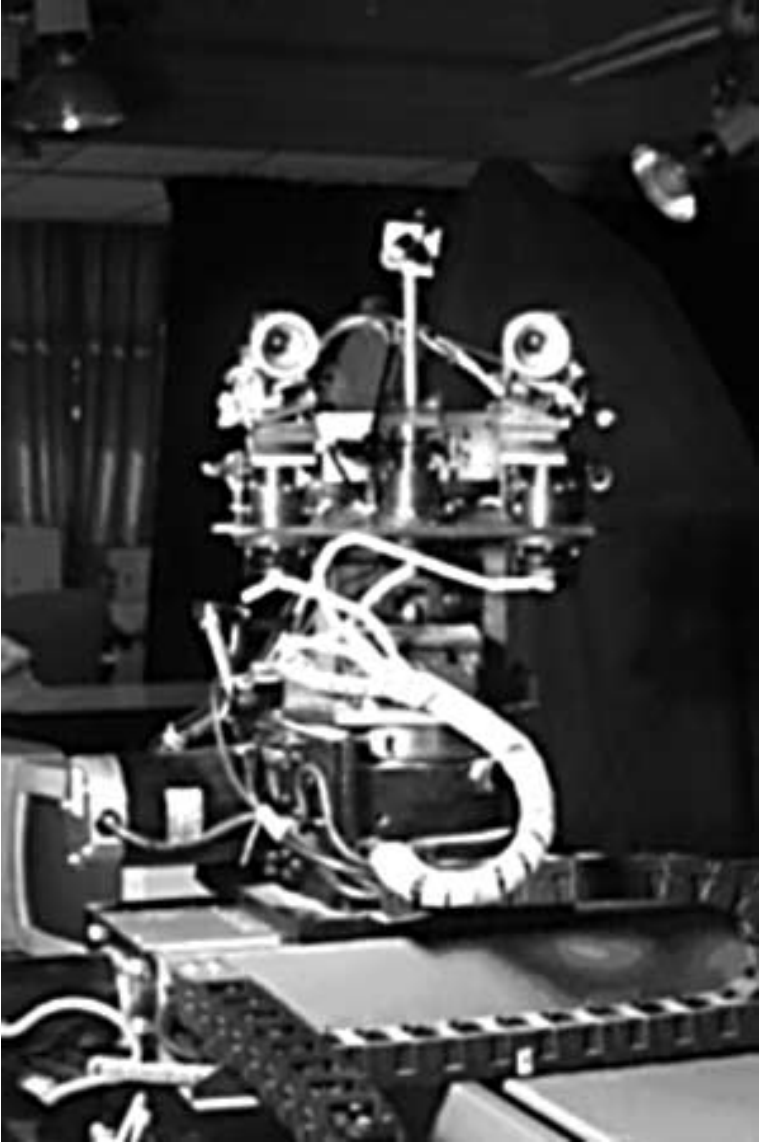
FIG. 7. The active binocular head (the IIS head) used in the experiments.
