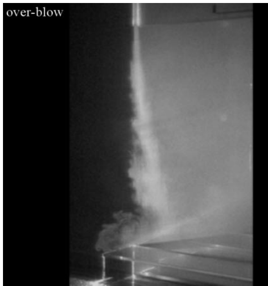
Fig. 6. Flow pattern of ‘over-blow’ air curtain at V_s = 3 \text{ m s}^{-1} , V_b = 6 \text{ m s}^{-1} , H = 60 \text{ cm} .
