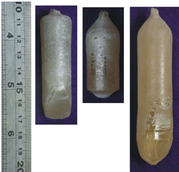
Fig. 2. As-grown SLN single crystals by the ZLCz method. Crystals from left to right are the 1st, 2nd, and the 3rd crystals grown from the same solution zone; the growth speed was 0.3 mm/h for the 1st and the 2nd crystals and 0.6 mm/h for the 3rd crystals.
