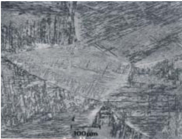
Fig.12. The microstructure of the Ti-6Al-4V alloy after rolling at 1000 °C.
