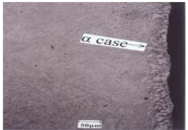
Fig.9. The microstructure of the Ti-6Al-4V alloy after holding for 1hr at 1000
