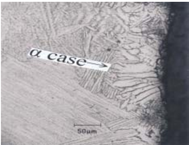
Fig.4 The as-cast microstructure of the Ti-6Al-4V alloy.
