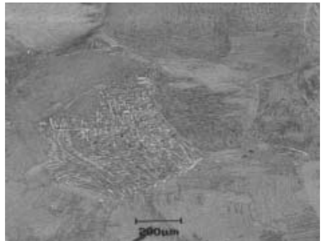
Fig.5 The as-cast microstructure of the Ti-6Al-4V alloy that was annealed at 900 for 1hr.
