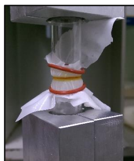
Figure 2-4 (A) Digital force gauge. (B) Procedure of testing the detachment stress of hydrogel by using egg membrane.
