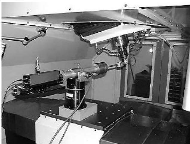
Fig. 5. Measuring the spindle with 3D LBB.
