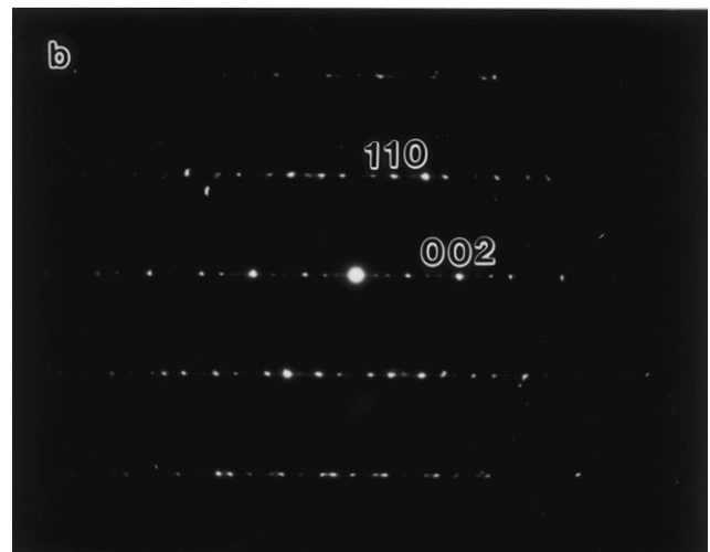
Fig. 9. (a) TEM bright-field image of Ti_{40.5}Ni_{49.5}Zr_{10} alloy aged at 300^\circ C for 240 h. (b) SADP taken from area E in (a), showing (001)_M compound twins with [110]_M zone axis.
