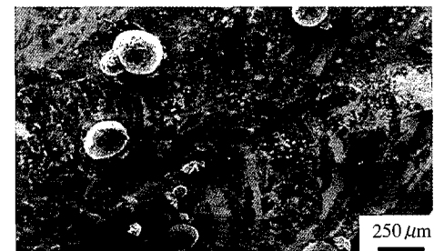
(c) 10%WC + Stellite12 coating (before wear test)
