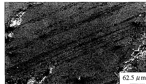
(d) 10%WC + Stellite12 coating (after wear test)
