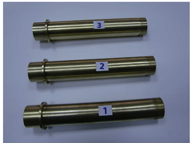
Fig. 9 – Photograph of the tested conical-cylindrical mixing chambers 1, 2 and 3.
