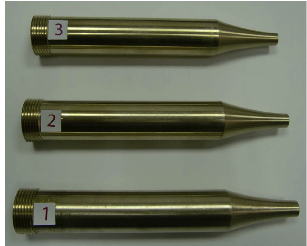
Fig. 7 – Photograph of the tested supersonic nozzles 1, 2 and 3.
