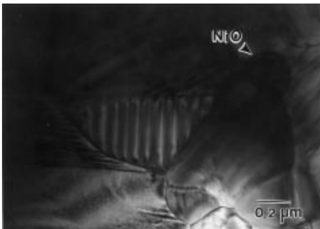
Fig. 9. A TEM micrograph of the 1.3 wt% NiO-doped BaTiO 3 specimen. The specimen is sintered at 1330 °C.
