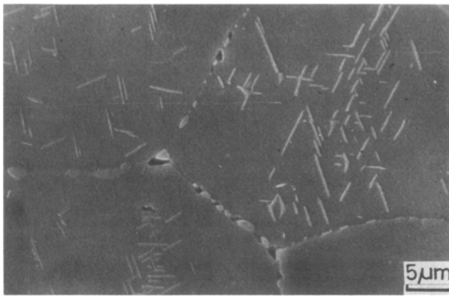
Fig. 3—Microstructure of the precipitated particles formed in the \text{Ni}_{78}\text{Al}_{21}\text{Zr}_1\text{B}_{0.2} alloy after air exposure at 750 °C for 500 h.
