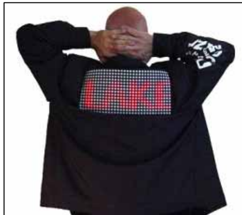
Fig. 1. Demonstration of a wearable flexible display powered by a wearable flexible solar cell.
