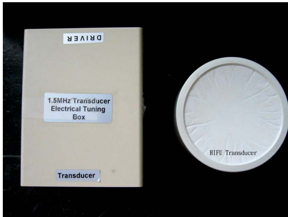
Fig. 4. The home-made HIFU transducer with ZrO 2 -epoxy matching layer.
