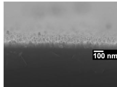
Fig. 5. SEM image of Ge-on-Si nanostructure.
