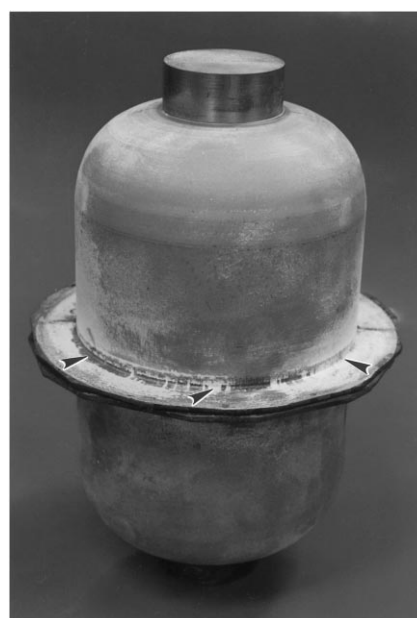
Fig. 10. Ti-6Al-4V high pressure vessel made by SPF/laser-welding, used to fill coolant for soldier-carrying infrared detectors. The laser weld line is indicated by arrows.
