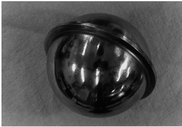
Fig. 11. Ti-6Al-4V spherical coolant containers for infrared detectors made by SPF/DB, used in middle-range missiles.
