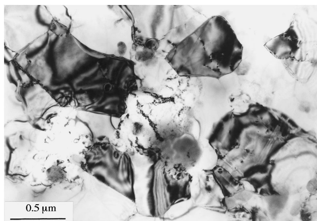
Fig. 3. TEM micrograph showing the (sub)grain structure of the LTSP 8090 Al sheet before SP loading, seen from the rolling plane. The (sub)grain shape was not completely spherical with a dimension of \sim 0.7 \times 0.5 \times 0.2 \mu\text{m} . After SP straining to \sim 50\% , the grains gradually become equiaxial.
