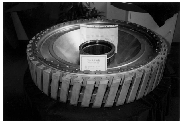
Fig. 20. The hollow fan hub made from Ti-6Al-4V forged rings, applying the DB technique for bonding a spacer (for dove tail and turbine fans) onto this hollow hub measuring 915 mm in outer diameter, 203 mm in inner diameter and 254 mm in thickness (courtesy of Shan-Tung aerospace company).
