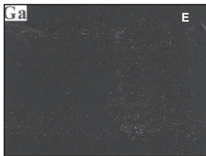
Fig. 4 — Micrograph and EPMA of the ITO/Cu joint soldered with Sn56Bi4Ti(Ce, Ga) active solder. A — The interfacial microstructure; B–F — elemental mappings of Sn, Ti, Ce, Ga, and O, respectively.
