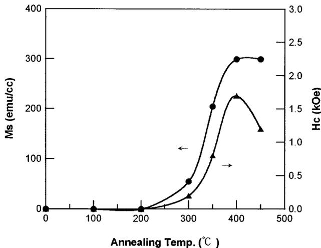
FIG. 4. Annealing temperature dependence of  $M_s$  and  $H_c$  for  $Mn_{50}Al_{50}/Al$  bilayer films.
