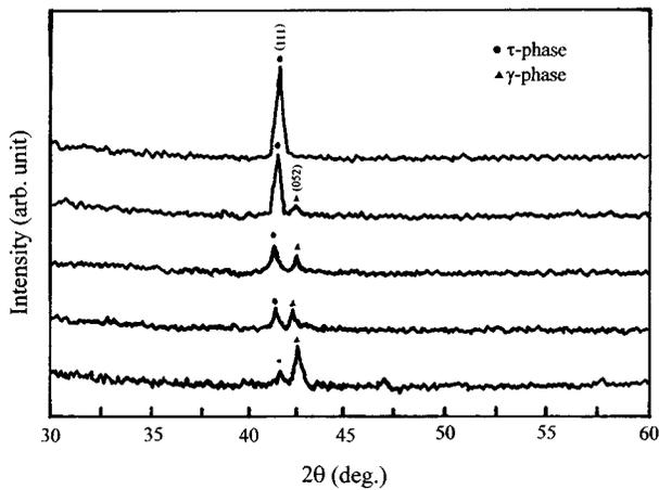
FIG. 3. X-ray diffraction patterns of  $Mn_{50}Al_{50}/Al$  films after annealed at 400 °C for 30 min, the thickness of Al layers are (a) 0 nm, (b) 30 nm, (c) 60 nm, (d) 90 nm, and (e) 120 nm, respectively.
