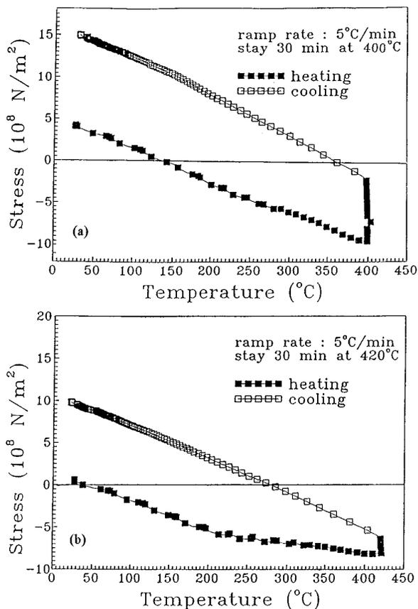
FIG. 6. Temperature dependence of stress for  $\text{Mn}_{50}\text{Al}_{50}/\text{Al}$  bilayer films, the thickness of Al layer is 30 nm. (a) Annealed at 400 °C for 30 min. (b) Annealed at 420 °C for 30 min.
