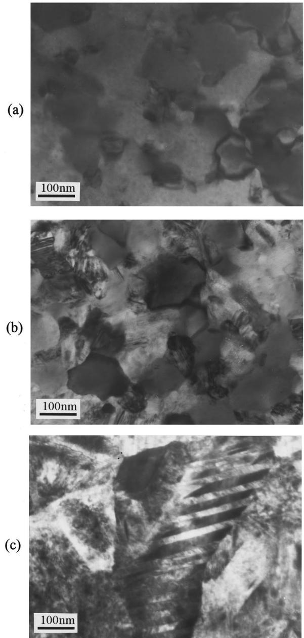
FIG. 5. The TEM photographs of the films annealing at (a) 100 °C, (b) 300 °C, and (c) 400 °C for 30 min.
