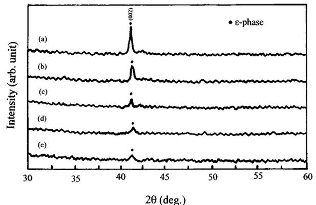
FIG. 1. X-ray diffraction patterns of as deposited Mn<sub>50</sub>Al<sub>50</sub> films with thickness of 600 nm, the thickness of Al underlayer are (a) 0 nm, (b) 30 nm, (c) 60 nm, (d) 90 nm, and (e) 120 nm, respectively.
