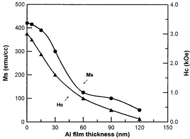
FIG. 2. Magnetic properties of  $Mn_{50}Al_{50}/Al$  bilayer films with various thickness of Al layer after annealed at 400 °C for 30 min.
