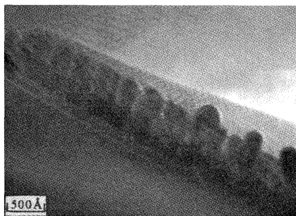
Fig. 1 TEM crosssection image of an [\text{Fe}_{50}\text{Co}_{50}(15\text{Å})/\text{Ag}(37\text{Å})]_{12} film annealed at 200 °C.
