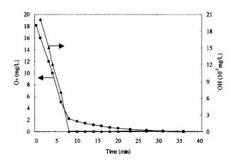
Fig. 7. Measured concentration of dissolved ozone and hydroxyl radical during the  $O_3/UV$  process
