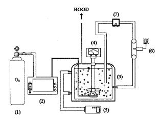
**Fig. 1.** Experimental apparatus of the ozone batch reactor: (1) oxygen cylinder; (2) ozone generator; (3) batch reactor; (4) 6-bladed-disk turbine; (5) thermostat; (6) pH meter; (7) pump
