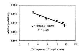
**Fig. 6.** Correlation between hydroxyl radical exposure and residual alkalinity ratio at pH 9
