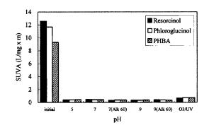
**Fig. 9.** SUVA measured at various levels of pH and alkalinity for model compounds treated by the ozonation and  $O_3/UV$  processes
