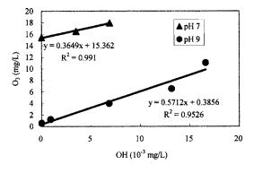
**Fig. 4.** Relationship between ozone and hydroxyl radical concentration at pH 7 and 9 in the ozonation process
