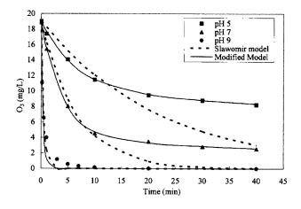
**Fig. 2.** Ozone decomposition and predictive decay model at different pH levels
