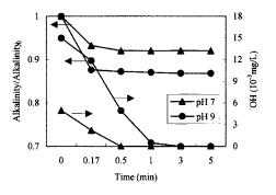
**Fig. 5.** Correlation of residual alkalinity ratio and hydroxyl radical concentration during the ozonation process
