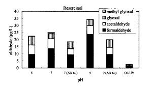
Fig. 10. Formation of aldehyde for resorcinol at various levels of pH and alkalinity treated by the ozonation and  $O_3/UV$  processes
