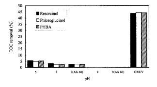
**Fig. 8.** Removal of TOC at various levels of pH and alkalinity for three model compounds treated by the ozonation and  $O_3/UV$  processes
