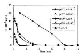
**Fig. 3.** Difference in hydroxyl radical between ozonation and O<sub>3</sub>/UV processes
