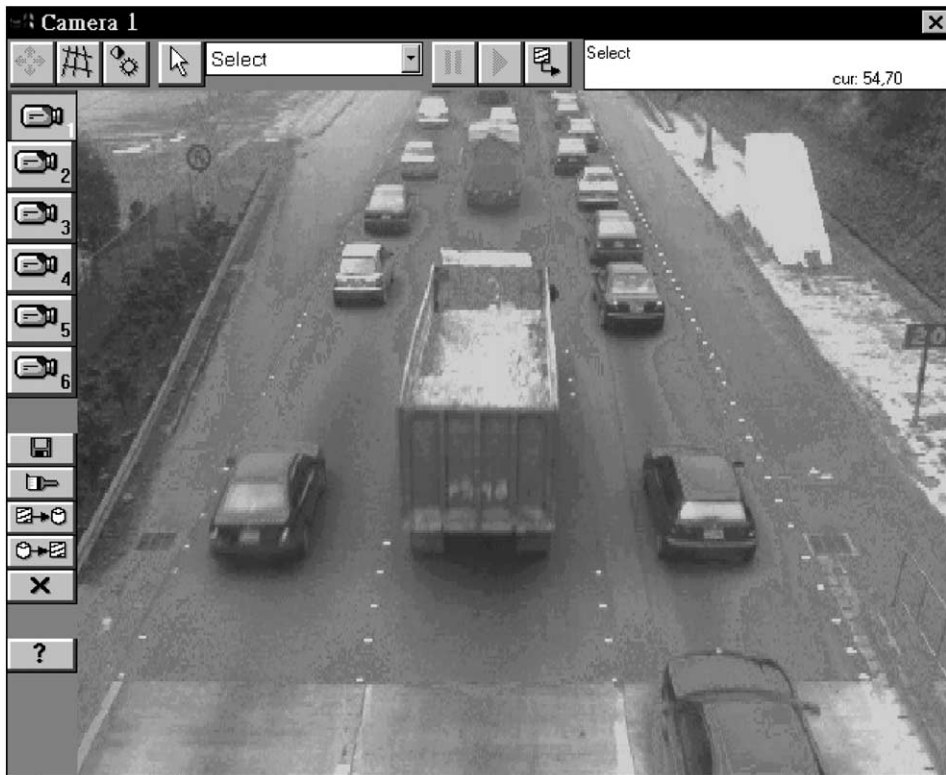
Fig. 2. The view of the CCD camera, which shows the traffic at the outlet portal of the southbound tube of Fu-De Tunnel at 8:04, 2000/4/13. One detection zone is defined for each lane in the image-process system. The cargo truck and the two sedans on the two sides happened to be in the detection zone of each lane. The speed and the length of each vehicle and the number of vehicles passing through each detection zone are measured and recorded chronologically.
