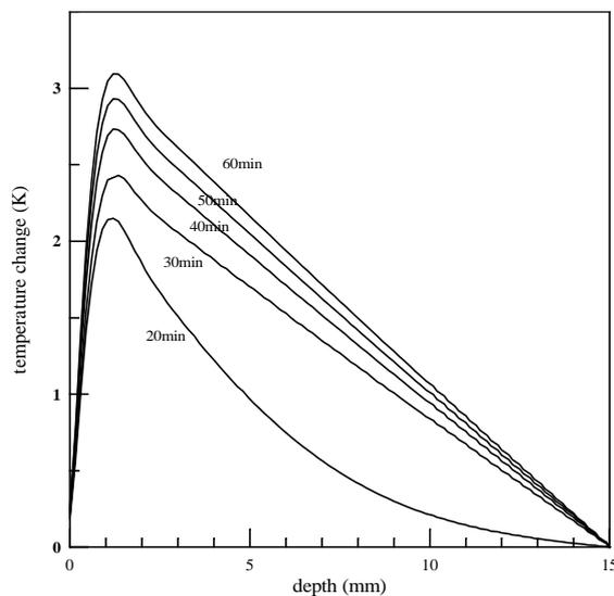
Figure 1. Temperature-distance profile in the UHMWPE component for five different walking times.
