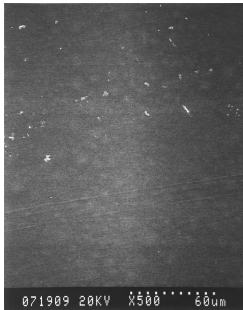
Fig. 6. The surface morphology of a dense PLLA membrane prepared by directly evaporating a casting solution of 20 wt% PLLA.
